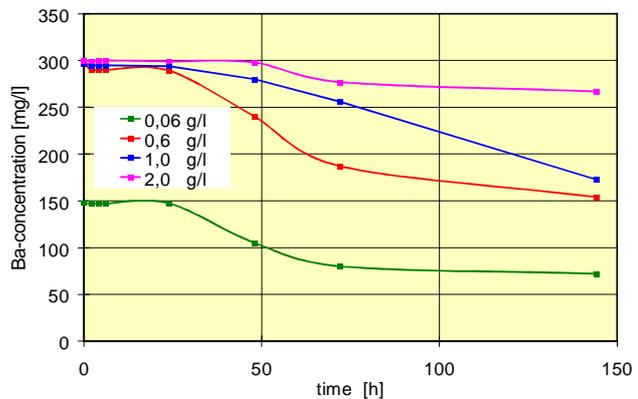
Fig. 2: Course of BaSO<sub>4</sub> precipitation depending on the inhibitor concentration
