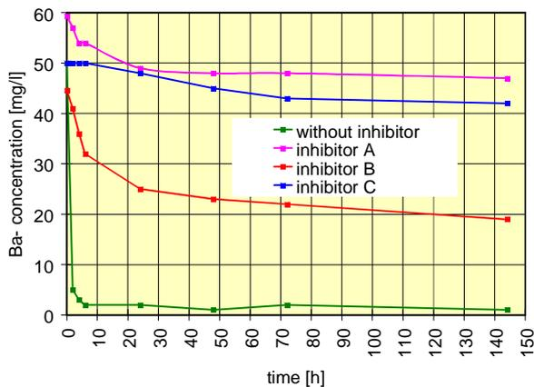
Fig. 1: Course of BaSO<sub>4</sub> precipitation depending on the used inhibitor
