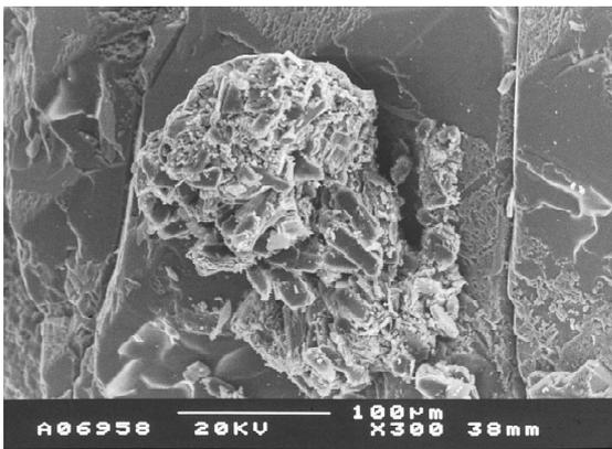
Fig. 3: SEM picture of BaSO<sub>4</sub> layers grown on sandstone.
