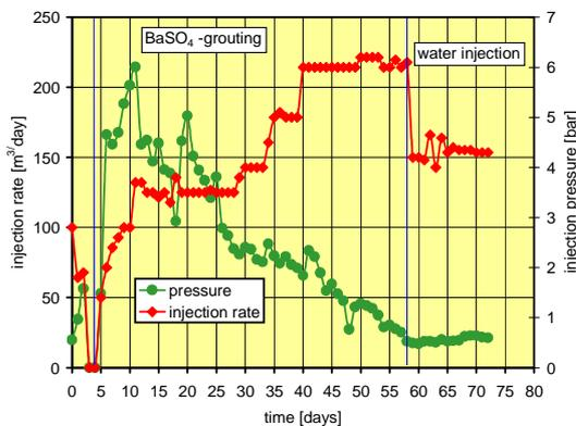
Fig. 5: Development of injection rate and pressure
